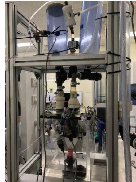
**Pro-05: Improved in-vitro testing of a suture-less inflow cannula using a bioreactor**
